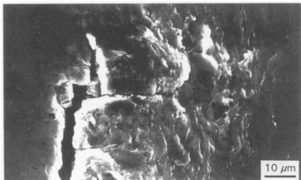
Figure 5 Plastic deformation and microcrack forming at a crack tip in the unreinforced alloy at high \Delta K values.
